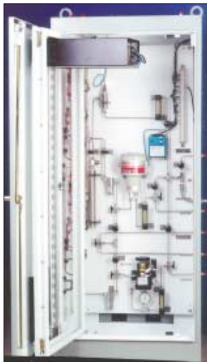
Fig. 7 — Sampling systems extract, cool, and clean furnace atmosphere samples. The system must not add or remove water vapor from the dew point test gas. For many furnaces, a turnkey sampling system having sensors for oxygen and other process parameters in addition to those for dew point might be appropriate.
