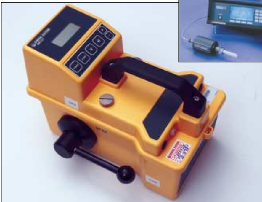
Fig. 5 — A variety of metal oxide trace moisture instruments are used in heat treating applications. They include integrated transmitters, top; analyzers with remote probes, inset; and portable battery-operated hygrometers, bottom.
