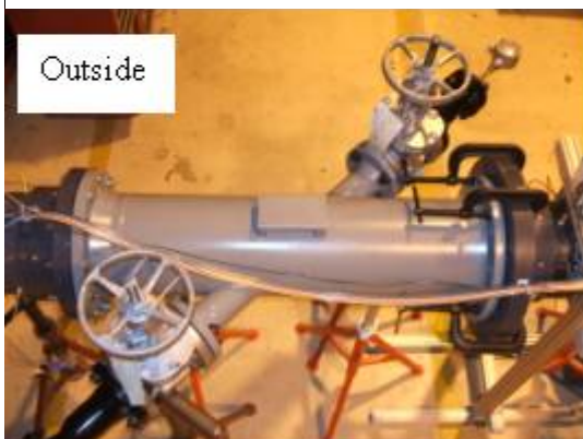
Figure 6 (b). Pictures of the Diagonal 45 carbon steel flowcell with transducers mounted, outside and inside views.
