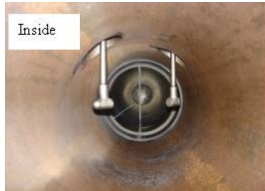
Figure 6 (a). Pictures of the Bias 90 carbon steel flowcell with transducers mounted, outside and inside views.
