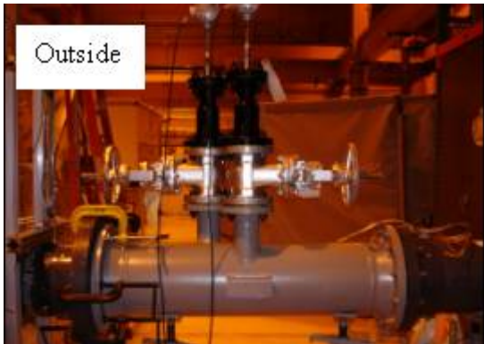
Figure 6 (a). Pictures of the Bias 90 carbon steel flowcell with transducers mounted, outside and inside views.
