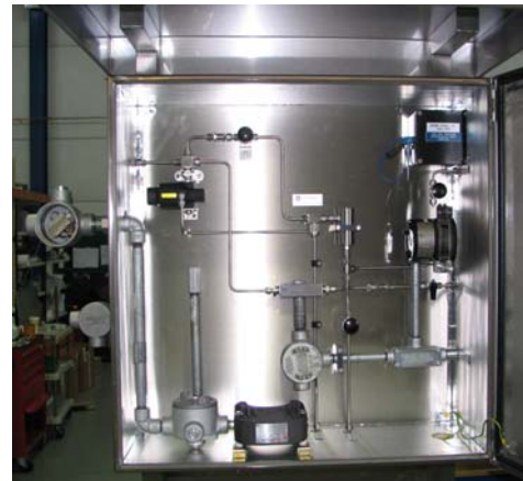
Example of moisture analyzer sample system panel for an aluminum oxide moisture sensor. The enclosure is insulated and an explosion proof heater (shown in bottom left of panel) is used to maintain temperature.
