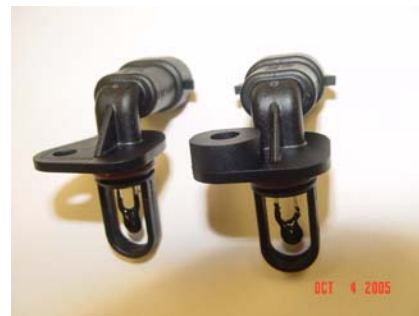
Figure 1: GE Sensing's Custom Designed Air Intake Manifold Sensors
