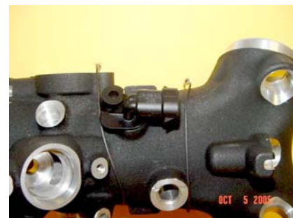
Figure 2: Air Intake Manifold Sensor Installed in Engine Manifold
