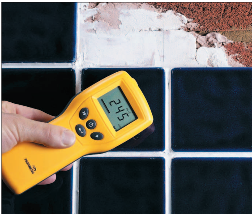
Protimeter's moisture measurement tool in action. The most credible way to diagnose the cause of any moisture-related problem is by measuring and monitoring moisture levels in the building.
