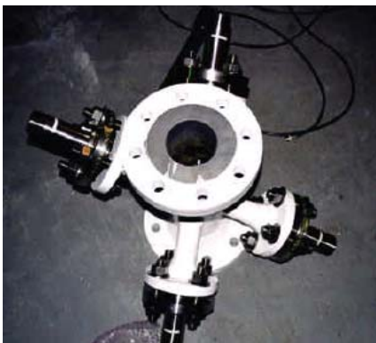
Meter body with BWT system showing redundant path configuration
