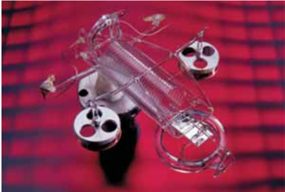
Series 7252s features a unique fused-quartz sensor. This rugged transducer offers unequalled precision and a stability of 0.0075% of reading per year.
