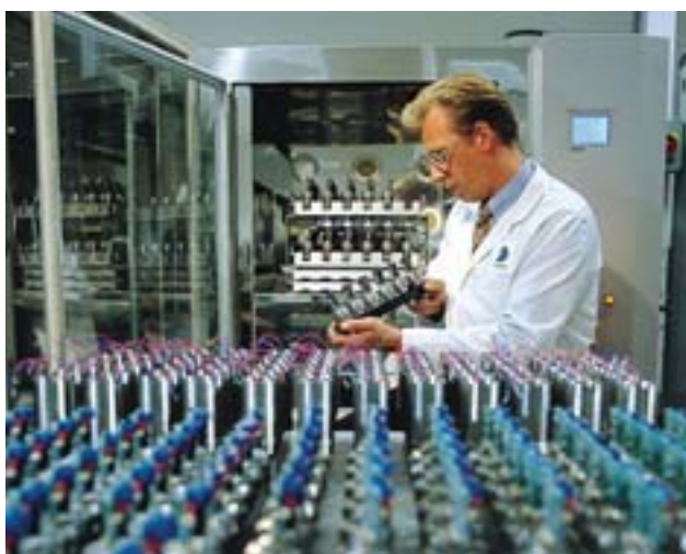
Computerised testing and calibration of pressure transducers.
